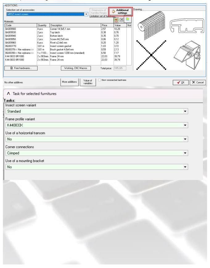
3. An exemplary view of the MRSZ insect screen with default settings, added to the tilt&turn window in the MB-86N system.
